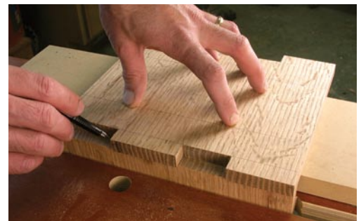
A little tracing. Use the cuts on the sides to mark the shape on the ends.
