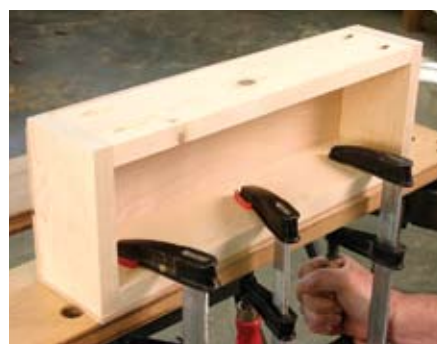
The aesthetics of the drawer, which shows no screws during normal use, is achieved by turning the pocket screws toward the outside of the drawer box and covering the front with the drawer face. Cut the face oversized and trim flush with your plane.
