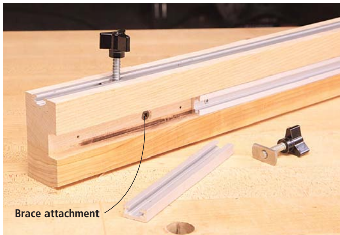
Install the T-slot tracks in the grooves with flat head screws countersunk into the track. The braces are attached to the fence by screwing through the face groove prior to attaching the T-slot track.
