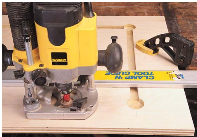
The grooves for the T-slot track allow the fence to be used left-to-right and front-to-back on the table to take advantage of the tilting feature of the existing table.
