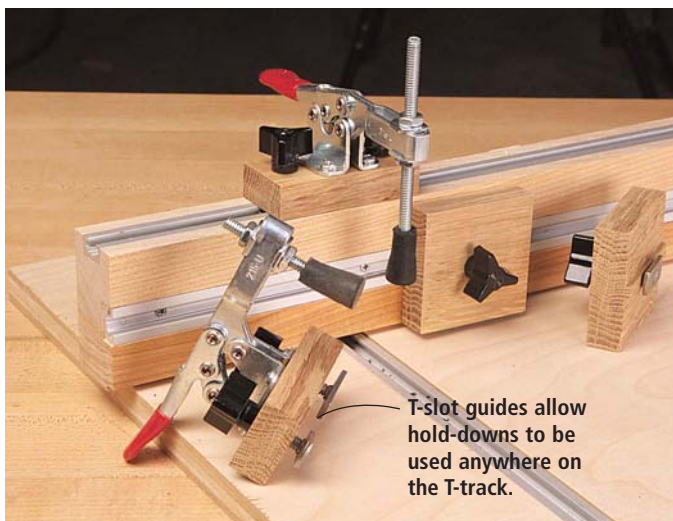
The hold-downs and stops are made from \frac{3}{4} " hardwood. To make the guide that holds the stops squarely on the fence, cut a \frac{1}{16} " x \frac{1}{8} " rabbet on both sides of the inside face using your table saw.
