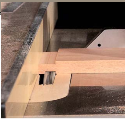
To cut the tenons, use a dado stack on the table saw. Reduce the tenon in thickness by \frac{3}{16} " on each side.
