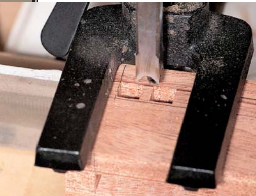
I made the mortises using a mortiser. In order to form the holes more safely, you should think of the path of least resistance. Instead of just going in a straight line from left to right or right to left, make two holes with a slight gap between. Then clear out the gap. If you simply work in a straight line, the mortiser's chisel could bend or break.
