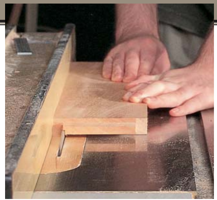
You will need to fasten the tabletop using tabletop fasteners, which requires making a kerf in the aprons. I made this kerf on the table saw \frac{1}{16} " from the edge and \frac{1}{4} " deep.
