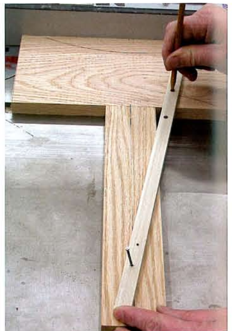
By using two steel rules in tandem I'm able to measure the actual required length of the dowels by measuring to the bottom of the dowel holes.
