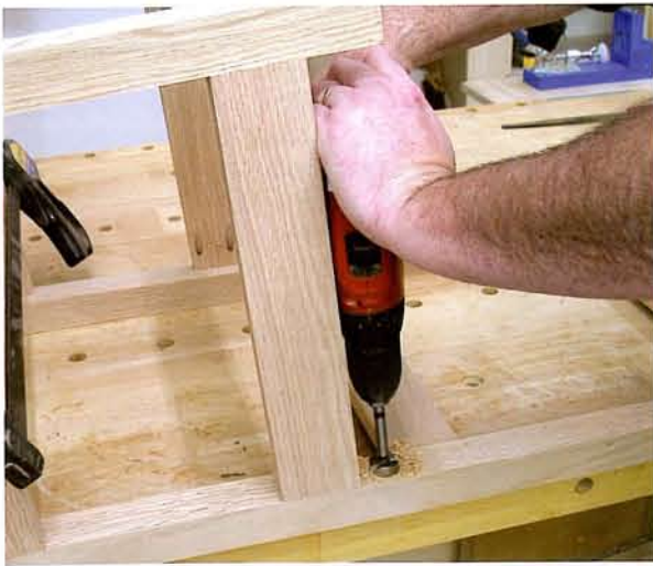
The dowel holes in the rear legs need to be drilled parallel to the side stretcher, not perpendicular to the rear leg, otherwise they just won't fit.
