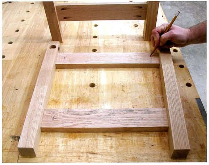
Laying the pieces for the side assemblies on your bench and marking everything will make sure you cut the pockets in the right places. Pencil lines are much easier to sand off than holes in the wrong location.
