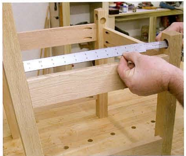
By using two steel rules in tandem I'm able to measure the actual required length of the dowels by measuring to the bottom of the dowel holes.
