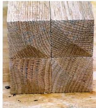
Set the miter saw to a five degree angle. Place the leg on the saw so that the cut begins about 1/2" down from the top of the leg. Use a stop block to hold the leg in place as you rotate the leg 90° to make the four cuts for each leg.
