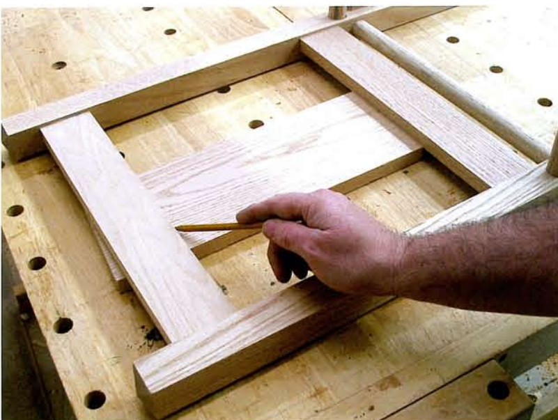
After marking the required length of the splat at the chair itself (above), use a home-made trammel to mark the curves to shape the splat (right).
