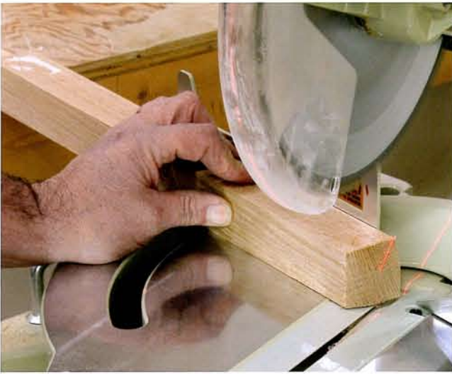
Set the miter saw to a five degree angle. Place the leg on the saw so that the cut begins about 1/2" down from the top of the leg. Use a stop block to hold the leg in place as you rotate the leg 90° to make the four cuts for each leg.
