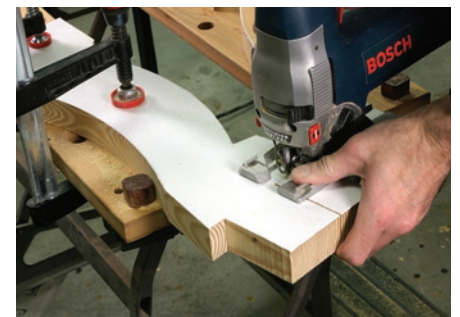
All in the jigsaw. The shape of and joinery on the legs is made entirely with a jigsaw. Follow close to the line and you won't have much cleanup work to do here.
