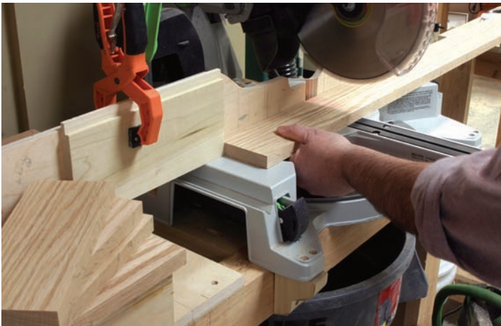
Consistent lengths. A stop-block and your miter saw work in unison to provide pieces that are equal in length – no matter the number of parts needed.
