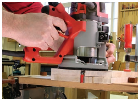
Exact replication. A flush-cut router bit with a top-mount bearing makes shaping the curves quick work, but the profile is only as good as the one copied.
