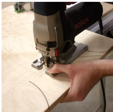
Angle of attack. Your jigsaw can't turn at sharp angles, so make a curved cut to the line.
