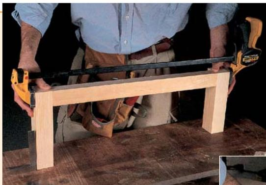
Be sure to make a full-size mock-up of the legs and sides (left) to determine the angle you need to cut on the bottom of the legs. When you determine that angle, use a grease pencil or magic marker to paint the bottom of the legs. I cut the back and front legs simultaneously. Slowly inch your legs in after each cut until the color is all gone (below).
