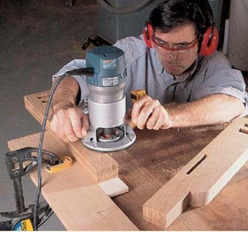
When pattern-routing the curve on the legs, make sure you have the work firmly clamped in place. I have the pattern and leg wedged between two pieces of oak (the pattern is on the underside of the leg). Then the leg itself is clamped to the table. You also could perform this operation on a router table with a starting pin for pattern-routing.
