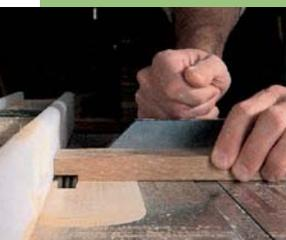
After you finish that first pass, slide the work against the fence and pull it back toward you over the blade to shave the last little bit of the shoulder.
