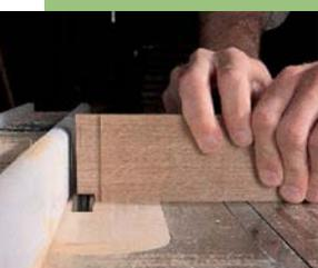
Repeat the same procedure for the edges of the tenon. (If you like a little more shoulder on your edges, increase the height of the blade.) First push the work forward.
