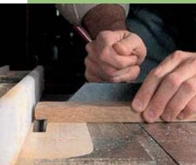
Set your fence so the dado stack will make a  $\frac{3}{4}$ " cut (the length of your tenon). Hold the piece about  $\frac{1}{8}$ " from the fence. Push your work through the blade using your miter gauge.
