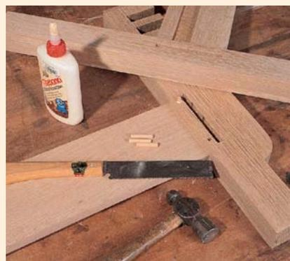
*Peg the tenons that join the front rail to the front legs and the back rail to the back legs. If you've ever pegged tenons before, you know that dowels can be wildly different sizes than they're supposed to be. Here's a trick. If your dowel is a bit undersized, glue it in place and cut it nearly flush to the surface. Then put several drops of thinned glue on the end grain of the dowel. It wicks in the glue, expands and glues up tight. When the glue is dry, cut the dowel flush.*
