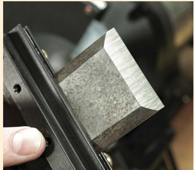
Your finished bevel should be even and straight across the blade.
