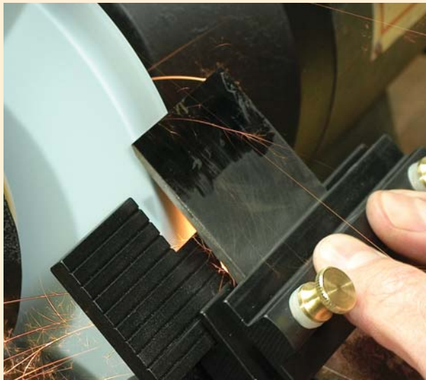
Avoid overheating while grinding the bevel.
