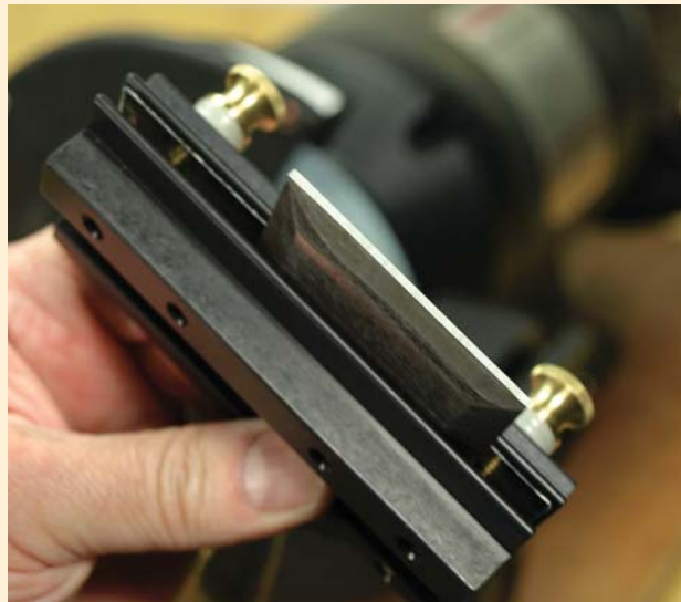
The edge is ground square across, ready for bevel grinding.
