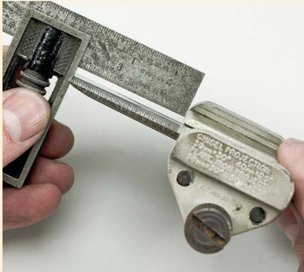
The distance from the guide determines the edge angle. This is a side-clamping, Eclipse-style honing guide.
