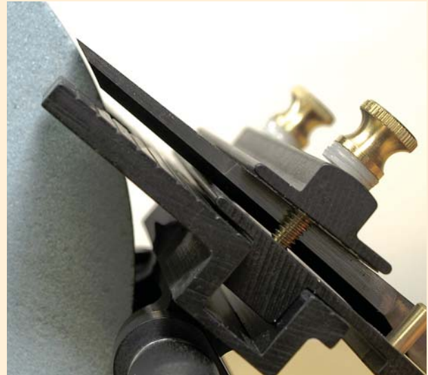
Establishing the bevel angle on a grinder requires a combination of blade extension and the articulation of the two joints of this Veritas grinder table.
