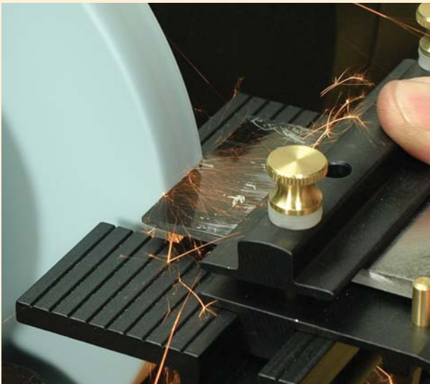
Grind to the line to remove nicks in the edge.
