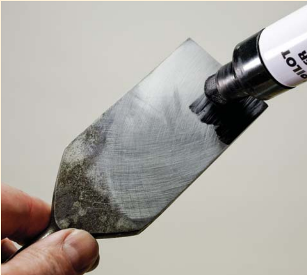
Use a felt-tip marker to color the blade for scribing.
