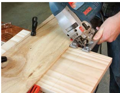
A jigsawn bevel. Set your jigsaw's baseplate to a 45° angle to cut the shelf to size.
