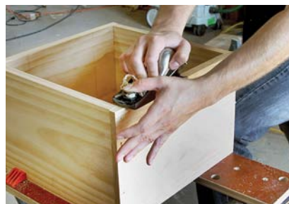
Trim up the edges. Dimensional lumber seldom results in perfect boxes – but a block plane can easily solve the problem.
