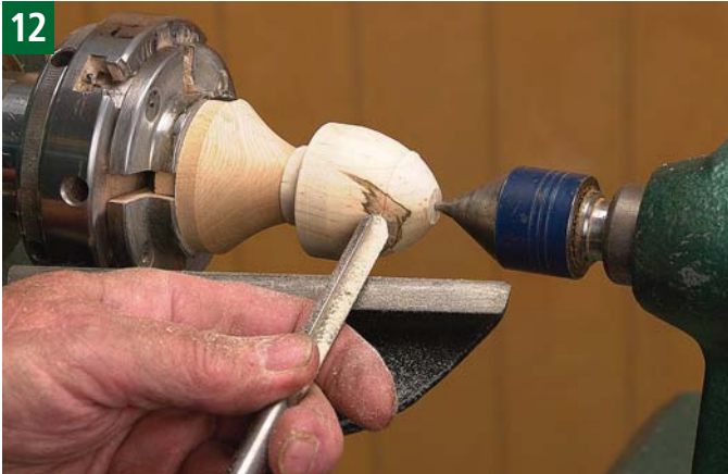
12 Move the tailstock and cone center in position to secure the body onto the mandrel. I use a \frac{3}{8} " spindle gouge for final shaping, cutting from the large to the small diameter with a light shearing cut.
