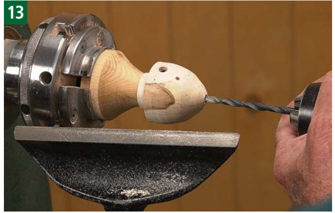
13 Drill a \frac{3}{16} " hole in the bottom of the body to hold the finial.
