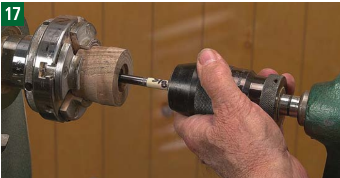
17 Select a block of wood for the roof. The procedure for roughing out the block and turning it to the required dimension is the same as shown in steps one through five for turning the body of the ornament. The only difference is the dimensions needed, and they are given on the drawing of the roof. For a basic roof, the block needs to be 1\frac{5}{8} " long and 1\frac{1}{8} " in diameter. Drill a 1" hole that's \frac{1}{8} " deep to provide a counterbore area for the top of the body to fit into. Now drill a \frac{5}{8} " hole that's \frac{1}{2} " deep to allow the top to fit on the wooden mandrel. This also removes some of the wood in the top, making it lighter. Sand and finish the underside of the top.
