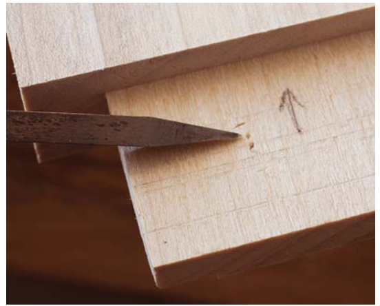
Here, not here. I moved the center point of the bore \frac{1}{16} " toward the tenon shoulder and marked it with an awl.
