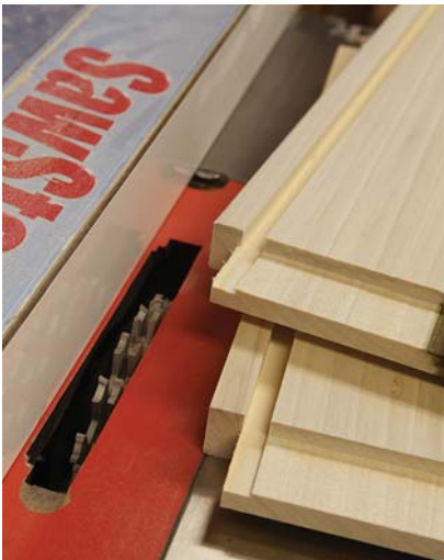
A groove for later. The groove in the top of the apron will hold the "buttons" that you'll screw to the underside of the base's top.
