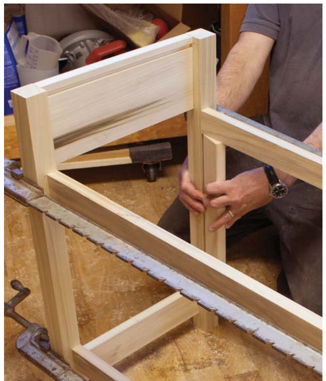
Like a door stile. If the stile is too long it won't fit in the table base. Cut it to a perfect fit before assembling the gate.
