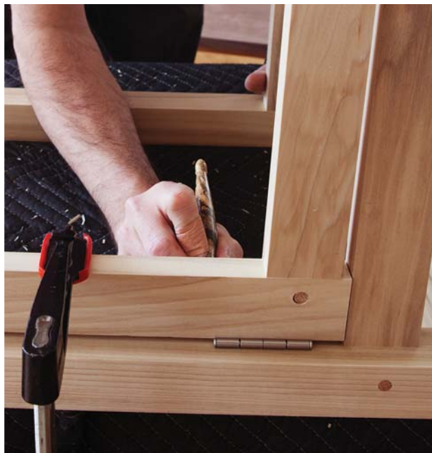
Clamp & knife. Put the gate in place and knife the location of the hinges on the leg.
