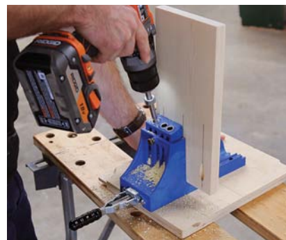
Pocket power. Carry marks up to over the jig top, then drill pockets at your apron ends.
