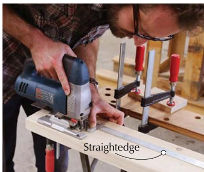
Leg rip. Use a straightedge as a saw guide and rip four 1 \frac{1}{2} "-square legs from the 2x6s.
