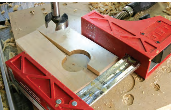
Can't-miss garter hole. Clamp the two halves of your garter together and bore the hole right through them. Our garter hole needed to be 1 5 / 8 " in diameter to match the dimension of the shaft of the vise's screw.
