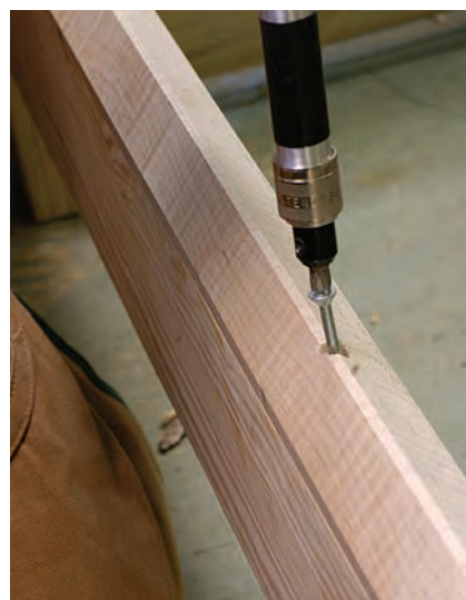
Resists dust. Some sliding jacks run in grooves that are plowed in the lower stretcher. These grooves fill with dust. By making the track for the board jack triangular in section, sawdust won't interfere with the movement.
