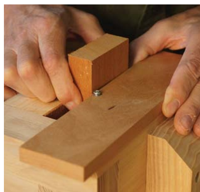
Perfect alignment. A disc (perhaps the round blade from a cutting gauge) screwed to a spacer block can help you to align your workpiece in the vise for dead-on sawing accuracy.
