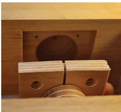
Fit to be screwed. Cut the recess for the garter in the vise jaw, then drill for and countersink for screws that will allow the entire assembly to move smoothly together.
