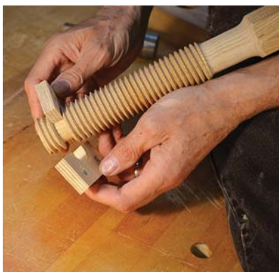
Handle it. After turning and threading the vise screw handle, fit the garter.
