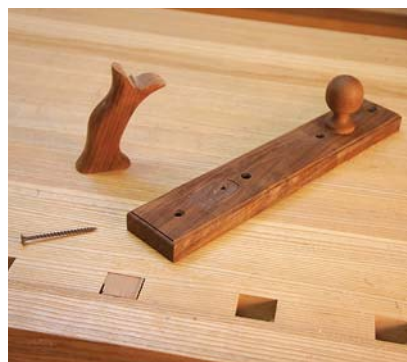
Parts. The saw consists of a blade, two blocks of wood, two handles and machine screws.
