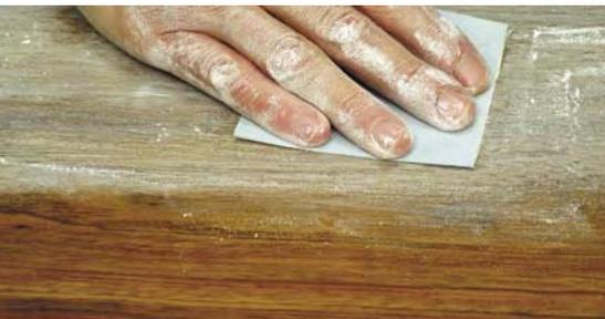
A varnish or lacquer sanding sealer has soap-like lubricants included, which make the finish powder when sanded. Sanding sealer reduces protection for the wood, however.
