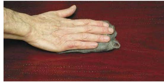
Instead of using steel wool dry, wet the surface with soap and water or mineral oil and then rub. Rubbing wet produces better results, but you run the risk of rubbing through and not seeing it happen. You will make the rub-through much worse.
