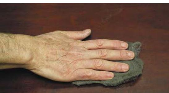
You can create a fairly smooth finish with an even sheen by rubbing with #0000 steel wool. Be sure to rub in the direction of the grain.
