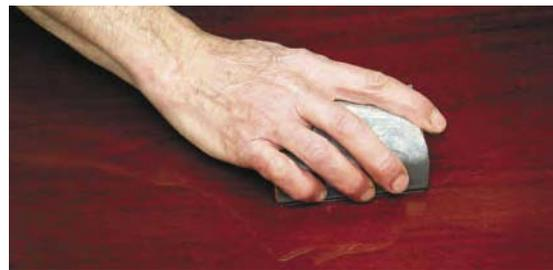
If you want to create the most perfect results when using a film-building finish, you have to level it using fine wet/dry sandpaper, a backing block and a lubricant.
