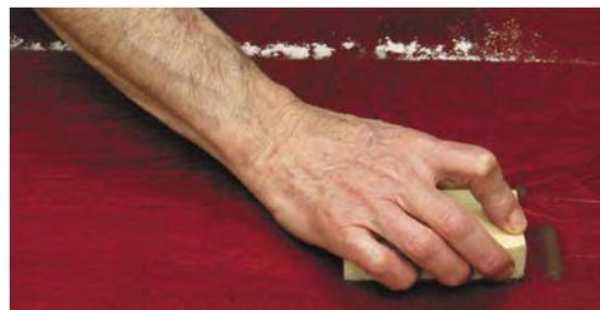
You can create an even satin sheen on a leveled surface by rubbing it with pumice and a mineral-oil or mineral-spirits lubricant. Use a felt or sponge pad.
