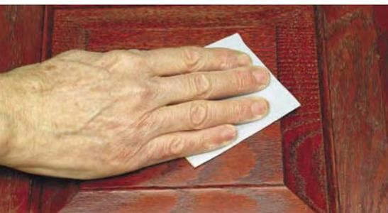
It's always best to sand between coats of a film building finish to remove dust nibs. Use steared sandpaper to reduce clogging.
