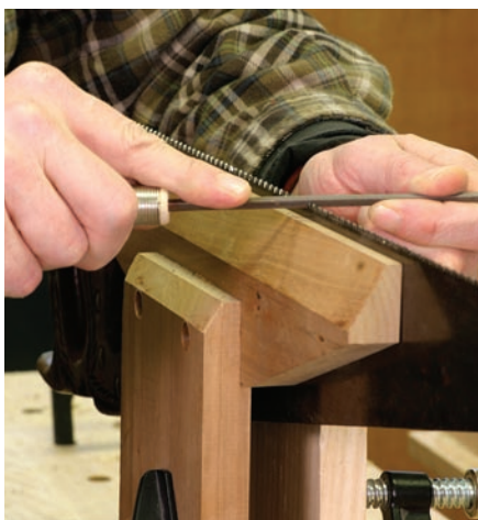
Tight fit. The jaws of the vise hold the sawblade and keep it from vibrating. If you hear an awful noise, the jaws need some work.
