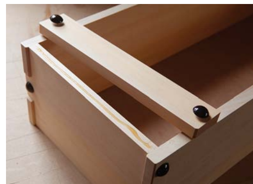
Here's the point. To prevent the battens from sliding around, drive the dome-head nails into each batten so the tips protrude just a bit. Add the glue. Then press the batten in place. The tips of the nails will prevent the batten from sliding.
