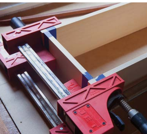
Tape & clamp. Painter's tape protects your planed surfaces from glue. Clamps press the corners tight.
