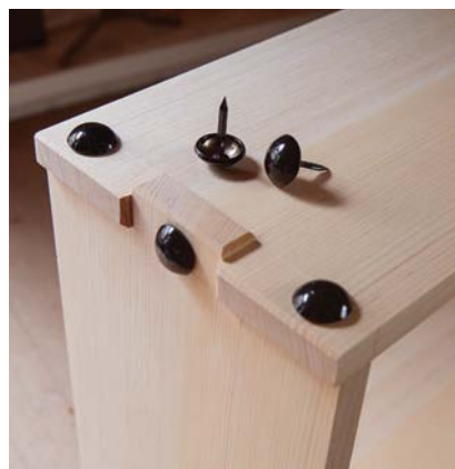
Decorative security. These dome-head nails don't hold as well as a cut nail, but they do add strength and prevent the wood from getting scuffed.
