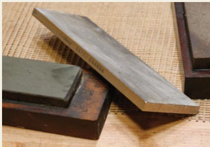
Oilstones. The term for these stones is a misnomer – they can be lubricated with water, soapy water, spit and other fluids.
