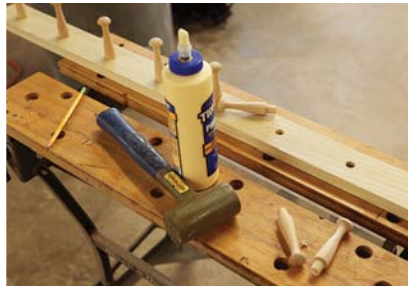
Pegs. A little glue and a light tap with a mallet to fully seat the pegs will keep things in place.
